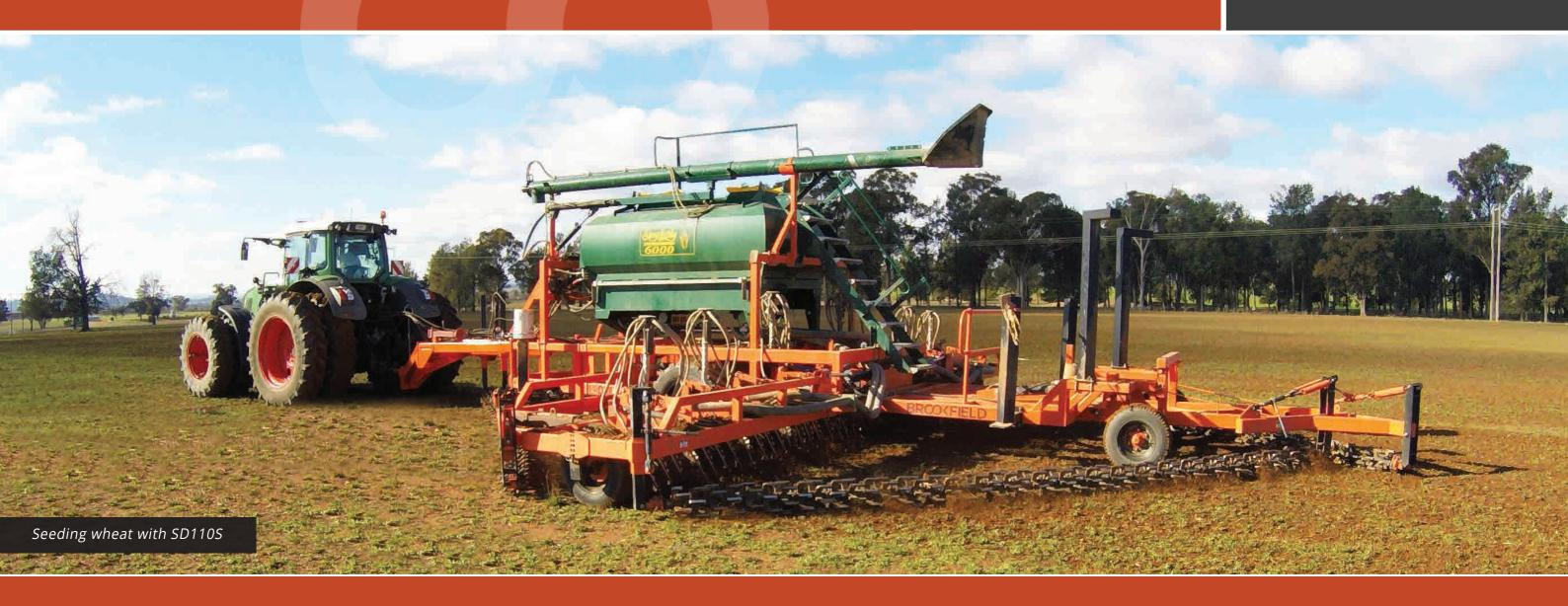
The BROOKFIELD<sup>®</sup> SUPERDRILL is fitted with gangs of 4-6 coulters at 250mm (10") spacing "standard" or the option of 200mm (8") or 300mm (12"). These 500mm (20") dia. coulters run on a 4<sup>o</sup> angle with a single bevel for maximum penetration and trash flow.
