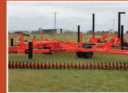
Creating a seedbed with sharpened disc DC90
