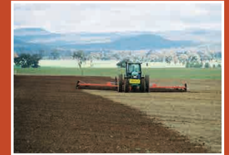
Creating a seedbed with sharpened disc DC90
